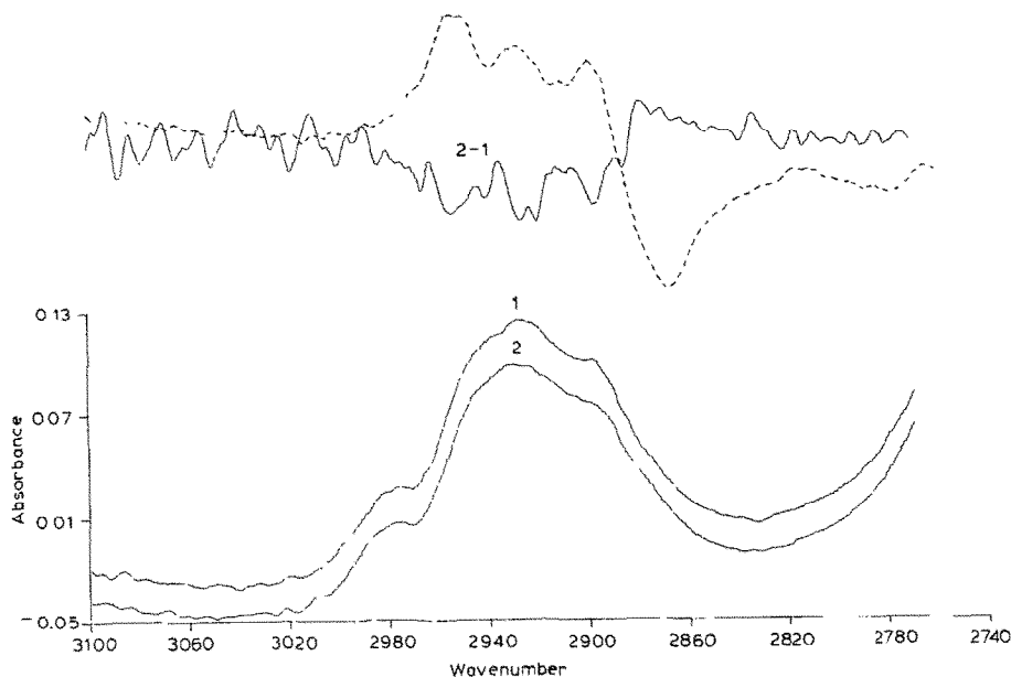
Fig. 1. F-t.i.r. spectra of L-lyxose in D_2O , with a starting composition of 95% of the \alpha anomer. [Trace 1 was obtained immediately after dissolving, and that numbered 2, after 1 h. The difference between the two is shown at the top. The dashed curve represents a similar difference for L-lyxose having a starting composition of 27% of the \alpha anomer].
